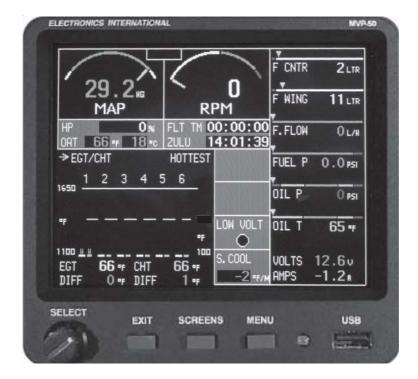
Figure 1, MVP-50 with Main Engine Screen
